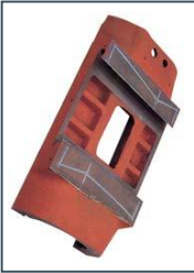
• Superior Turcite-B coated on the adjunction surfaces to the slideways and with precise scraping.
