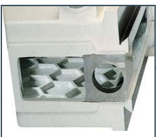
• High quality meehanite cast iron by resin mould then with annealing treatment to release stress, well designed inner structure, all for high strength and minimal deformation. Table and all slideways surface are harden and ground.
