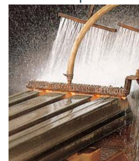
• High quality meehanite cast iron by resin mould then with annealing treatment to release stress, well designed inner structure, all for high strength and minimal deformation. Table and all sideways surface are harden and ground.
