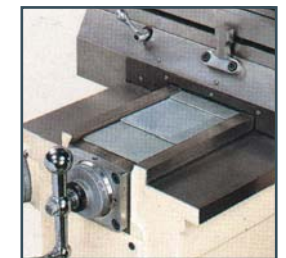
• ■ shape cross slide ways (For 2SLB, 3SB, 4S, 5S, 6S & 7S series)
