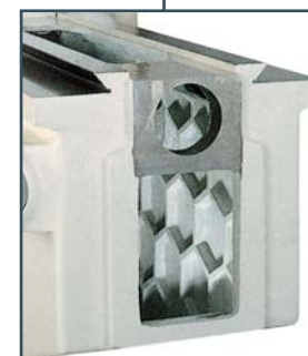
• High quality meehanite cast iron by resin mould then with annealing treatment to release stress, well designed inner structure, all for high strength and minimal deformation. Table and all sideways surface are harden and ground.
