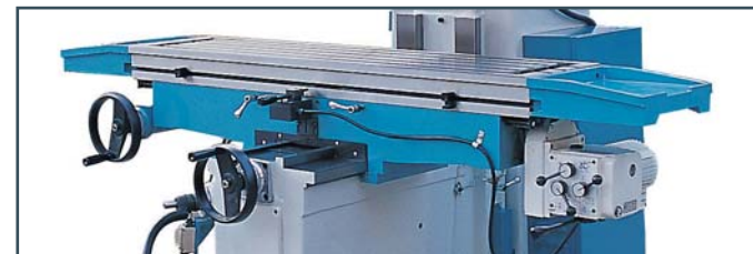
• Wide saddle structure with screw inside of it to have better support to the table (For 5S, 6S & 7S series)
