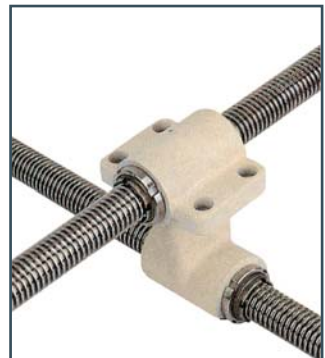
• Precise X & Y leadscrews features double nut compensator allow backlash to be eliminated.
