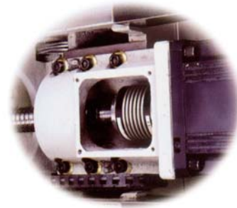
X/Y/Z axis transmission system by Germany precise direct drive connector
