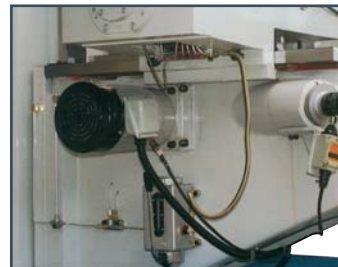
Outside motor driven Table Rapid elevating system (For Model: 5, 6, 7 & 8)
