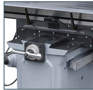
Double ▲ shape cross slideways (For Model X)
