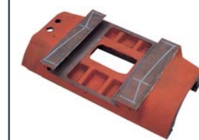
Superior Turcite-B coated on the adjunction surfaces to the slideways and with precise scraping.
