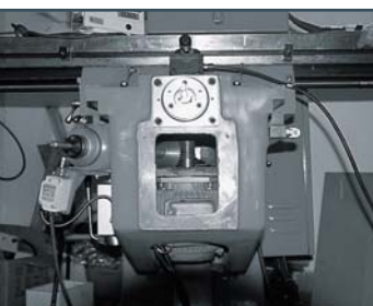
Inner Motor driven Knee Table Rapid elevating system (For Model: 4, 4L and X series)
