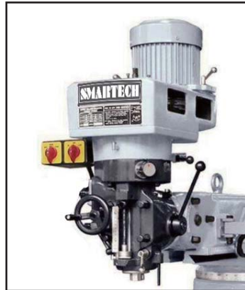
3J (3HP) Rigid Step-pulley.
