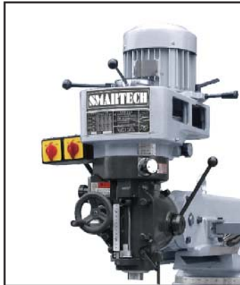
3S (3HP) Step-pulley.
