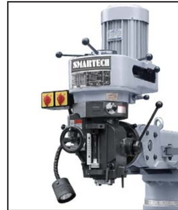
5S (5HP) Step-pulley
