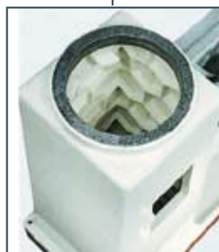
High quality meehanite cast iron by resin mould then with annealing treatment to release stress, well designed inner structure, all for high strength and minimal deformation. Table and all slideways surface are harden and ground.
