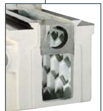
High quality meehanite cast iron by resin mould then with annealing treatment to release stress, well designed inner structure, all for high strength and minimal deformation. Table and all slideways surface are harden and ground.
