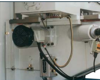
Outside motor driven Table Rapid elevating system (For Model: 5, 6, 7 & 8)
